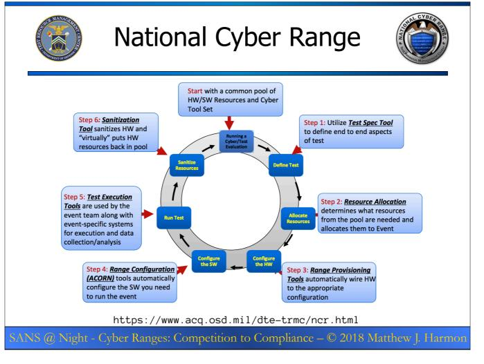
The Operational Procedures include hardware and software definition at the 12 O'Clock position, the expected results at 2 O'Clock then continuing clockwise we work through resource allocation, tool provisioning and configuration, range configuration loaded into the tool being tested, and then the actual test execution at 9 O'Clock including event specific simulations, finalizing with sanitizing of the environment and device being tested.
